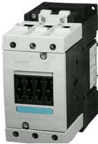
CONTACTOR, AC-3 30 KW/400 V, DC 24 V, 3-POLE, SIZE S3, SCREW CONNECTION
